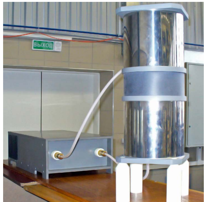
Fig. 1. Portable repetitive WB source with operation frequency up to 500 MHz
