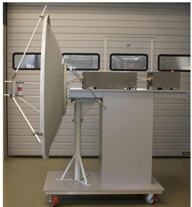
Fig. 5. Repetitive WB source with operation frequency of about 1GHz
